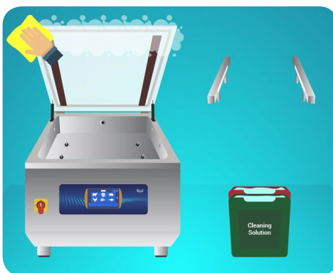
Using cleaning solution, clean lid, chamber, body, and under machine. Allow to air-dry.
