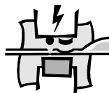
CUT-OFF SEAL 1 x 3,5 mm seal 1 x 1,1 mm cut single time setting
