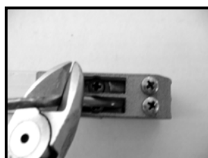
Pull wires taut using a pair of pliers and a vice and screw the wires down on the clamping plate.
