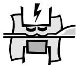
DOUBLE SEAL 2 x 3,5 mm seal
