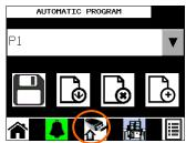
Press the "Program backup/restore" button and once the USB key has been inserted in the port behind the control panel, run "Backup" or "Restore" for the programs (recipes), following the displayed instructions.
