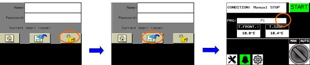
Once you have entered the "Name" e and the "Password" press these two buttons in the sequence indicated in order to access the display screens.
