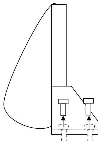
7. Loosen anchor bolt on torsion bar anchor assembly.
