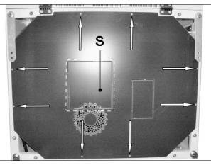
Fix support (8) to the cross member that supports the motor in the 4 holes indicated.
