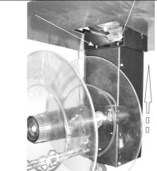
Fix the square (6) and the film guiding ring (5) to the machine through existing holes.
