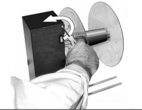
Position the machine, supporting it on one side so that you can remove the cover from the bottom, unscrewing the 8 fixing screws and detach the small square cover (S) using a tool (e.g. screw driver).
