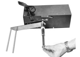
Fix the fixed flange (3) to the hub (2) using the 4 screws supplied.
