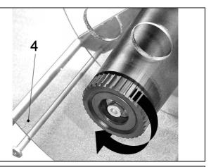
Disassemble the waste film rewinder case by loosening the 4 screws.
