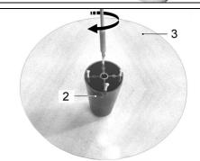
Place the hub with fixed flange on the rewinder shaft.
