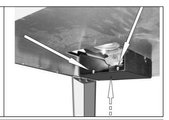
Fix the rewinder to support (8) and then replace and fix the rewinder guard.
